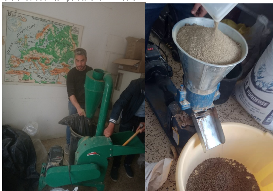
Production process of pellets
